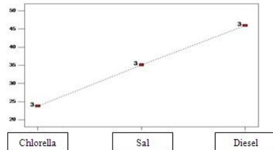
Figure 3: Heating value comparison of Microalgae methyl ester with Salicornia Methyl ester and diesel fuel
