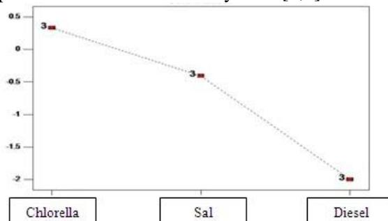
Figure 2: Cloud point comparison of Microalgae methyl ester with Salicornia Methyl ester and diesel fuel
