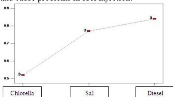
Figure5: Density comparison of Microalgae methyl ester with Salicornia Methyl ester and diesel fuel
