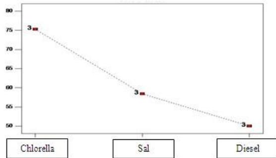
Figure 1: Cetane index comparison of Microalgae methyl ester with Salicornia Methyl ester and diesel fuel
