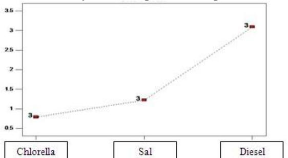
Figure 4: Kinematic viscosity comparison of Microalgae methyl ester with Salicornia Methyl ester and diesel fuel
