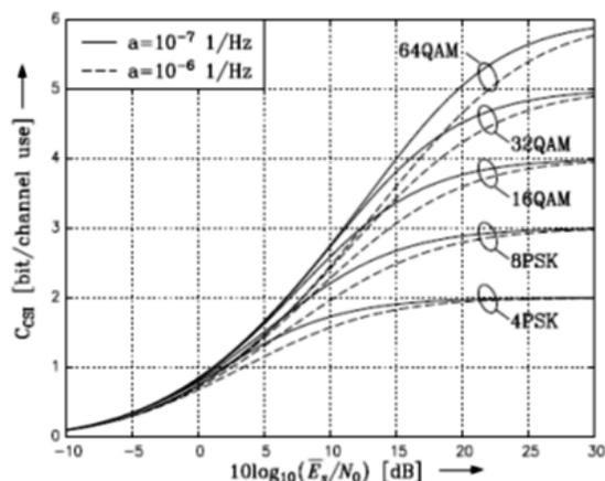
Fig. 7. Channel capacity for different modes
