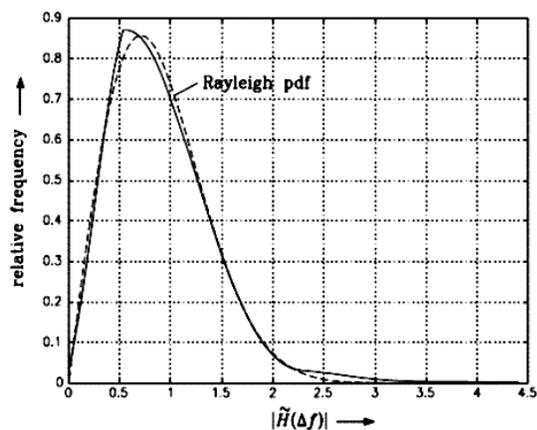
Fig. 6. Histogram of the normalized transfer function
