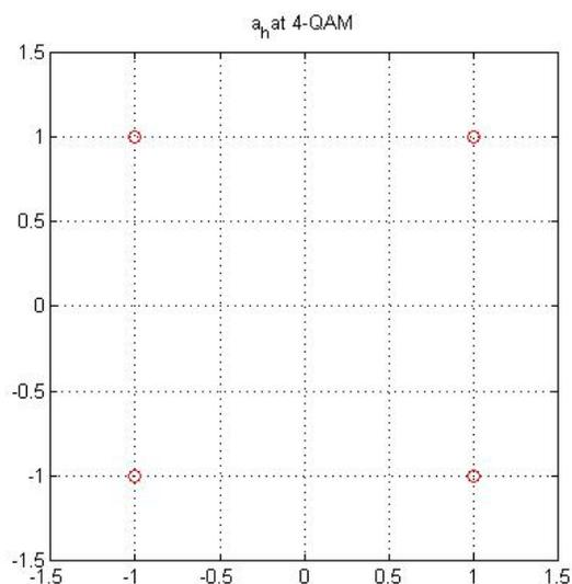
**Fig. 10.** 4-DAM modulation
