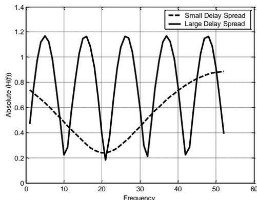
**Fig. 3.** Channel frequency response for the two-mode range with low latency and high
