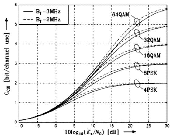
**Fig. 8.** Channel capacity for different conditions
