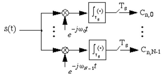
Fig2. OFDM demodulator
