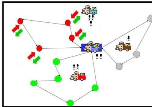
**Figure 1:** vehicle routing problem with regard to simultaneous pickup and delivery
