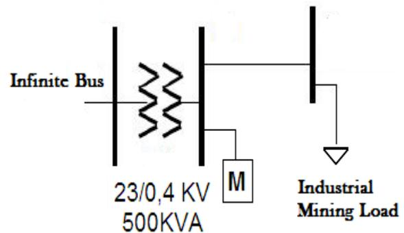
**Fig. 7:** Unilineal Diagram for Measuring and Recording of a Three Phase Test System
