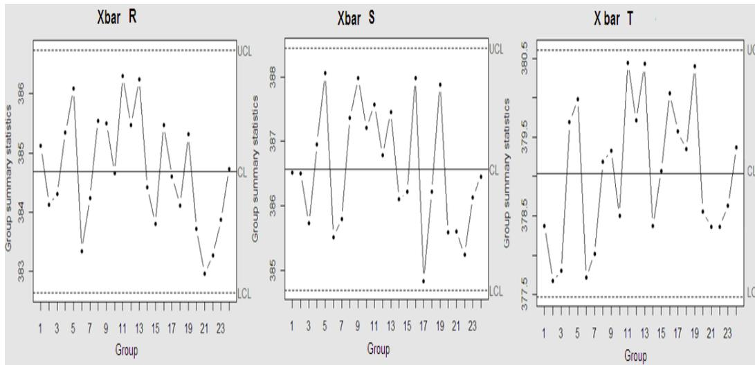
**Fig. 9:** Graph of XBar for R, S and T Phases
