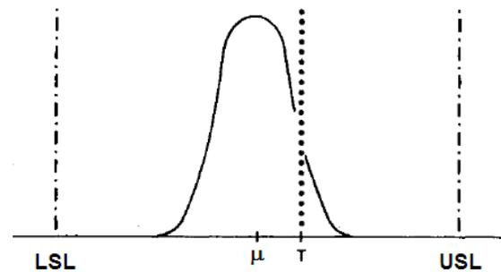
Fig.2 : Typical Graph for Process Capability Analysis
