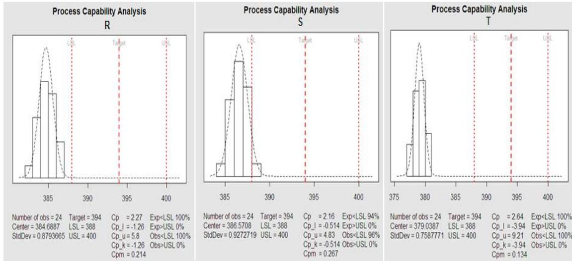
**Fig. 11:** Analysis of process capability for R, S and T phases
