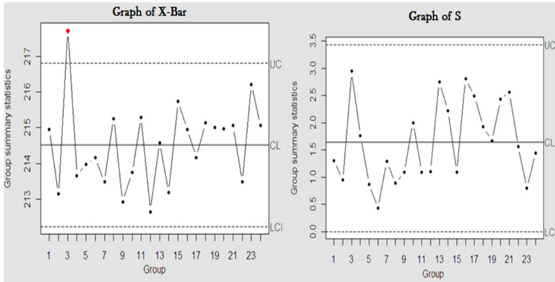
**Fig. 5:** Graph of Control XBar-S for Single Phase Sample
