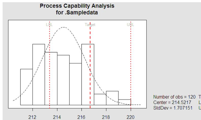
**Fig. 6:** Analysis of Process Capability for Single-Phase Sample
