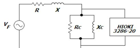
**Fig. 3:** Single Phase Circuit for Measuring and Recording
