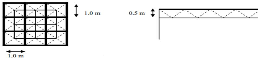
Walls of such frames, in addition to burdening vertical loads, are used as resistance systems in facing lateral loads and are made of one-way grids with rigid connections. In addition, the diagonal parts in walls are applied for bearing lateral loads.
