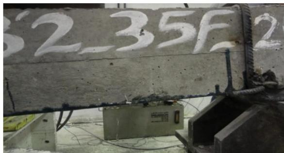
Picture 5 Anchorage in MSN cross bar in B2-F35-2L12.5 specimen
