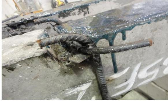
Picture 3 Bar anchorage with cross NSM bars
