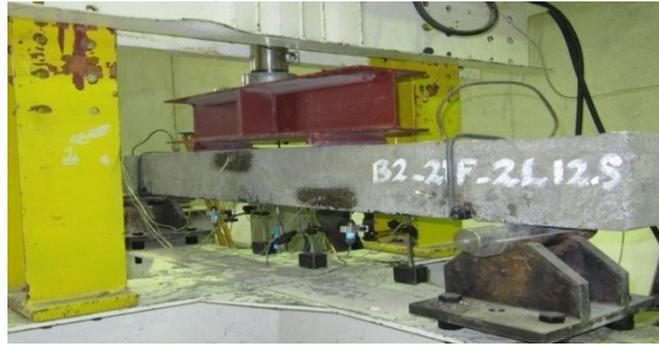
Picture 1 a four point flexural loading machine
