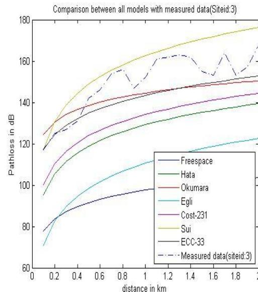
Figure 3 Comparative analysis of different path loss models with field measured data at Narnaul (INDIA)
