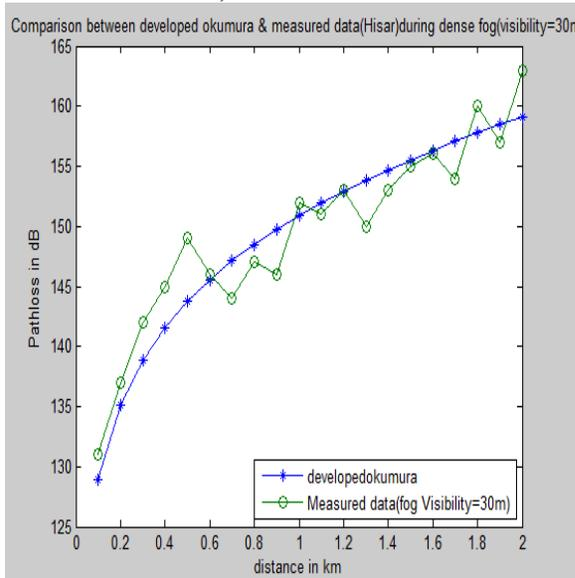
Figure 10 Comparison between developed okumura model and field data taken (Hisar, INDIA) in heavy fog condition
