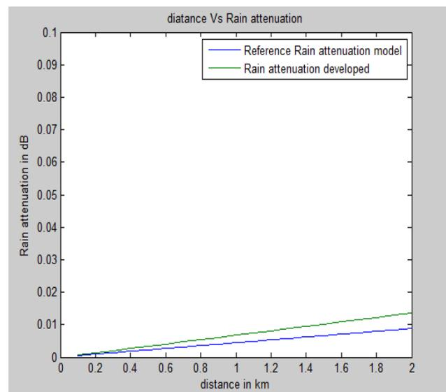
Figure 7 Comparison between developed rain attenuation and reference rain attenuation model
