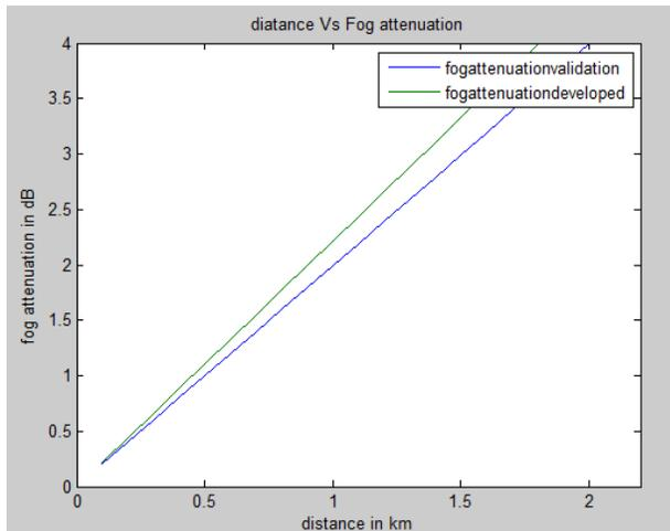
Figure 6 Comparison between developed fog attenuation and reference fog attenuation model
