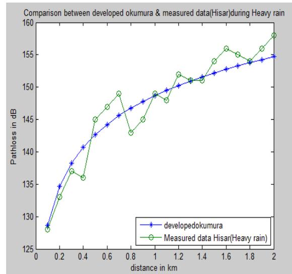
Figure 11 Comparison between developed okumura model and field data taken (Hisar, INDIA) in Heavy rain condition
