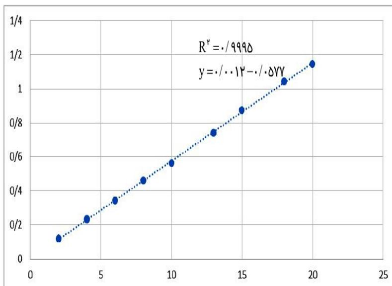
Figure 2: the graph of orange acid 2 **solutions** calibrations in 484nm
