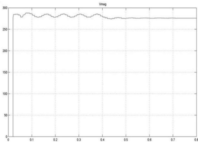
Figure. 5.1 Fundamental Voltage (Va) magnitude reduction and distortion without compensation (dead time = 10 μs)
