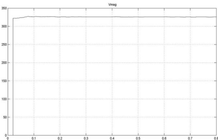
Fundamental voltage (Va) magnitude improvement after compensation (dead time = 10 μs)
