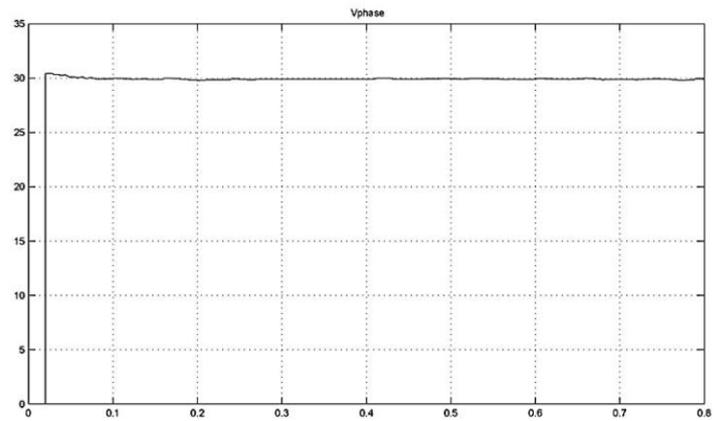
Figure. 5.3 Improved phase angle of fundamental voltage (Va) after compensation (dead time = 10 μs)
