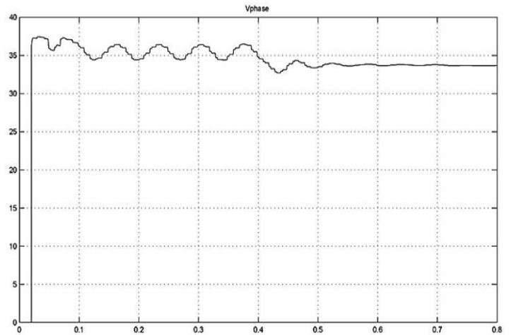
Figure. 5.3 Phase distortion of fundamental voltage (Va), without compensation (dead time = 10 μs)
