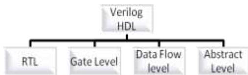
Fig. 02. Different programming modes in Verilog, HDL
