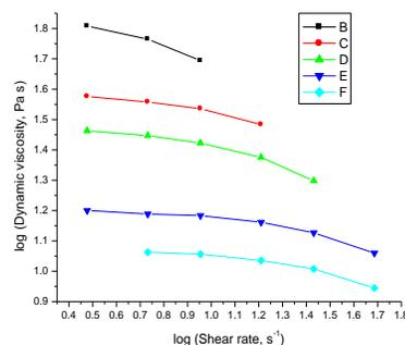
**Fig. 3.** Dependence log dynamic viscosity versus log shear rate concentrated solution 10 % at temperatures: B – 50°C, C – 60°C, D – 70°C, E – 80°C and F – 90°C
