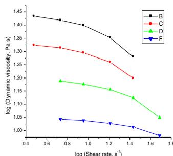
**Fig. 4.** Dependence log dynamic viscosity versus log shear rate 12 % solution concentrated at temperatures: B – 60°C, C – 70°C, D – 80°C and E – 90°C
