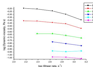
**Fig. 1.** Dependence log dynamic viscosity versus log shear rate of 3 % solution concentrated at temperatures: B – 40°C, C – 50°C, D – 60°C, E – 70°C, F – 80°C and G – 90°C
