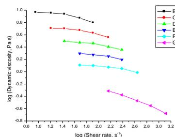
**Fig. 2.** Dependence log dynamic viscosity versus log shear rate of 6 % solution concentrated at temperatures: B – 40°C, C – 50°C, D – 60°C, E – 70°C, F – 80°C and G – 90°C
