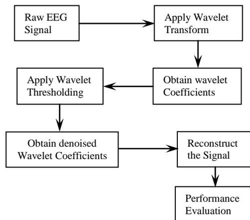
Fig 2. Denoising approach based on Wavelet Thresholding
