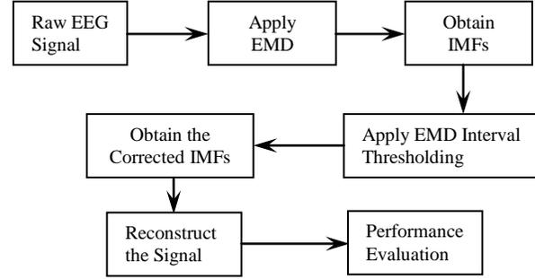
Fig 4. Denoising Approach Based on EMD-IMF Thresholding
