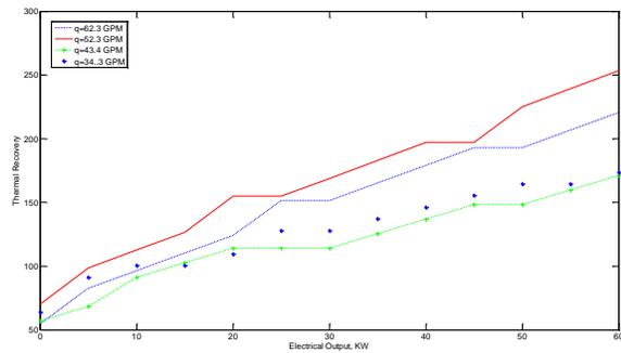
**Figure 6.** Thermal recovery of CHP generator at different loading and water flow condition
