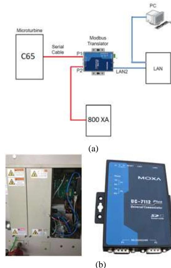
**Figure 3** Micro turbine of the MG communicating with DCS using Modbus protocol (a) typical connection diagram and (b) Modbus translator located at the back of Capston micro turbine [5], [9]
