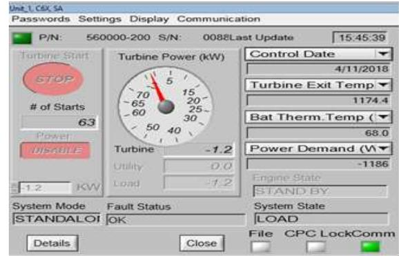
**Figure 7** CRM Control window for Generator control and selected acquired data display
