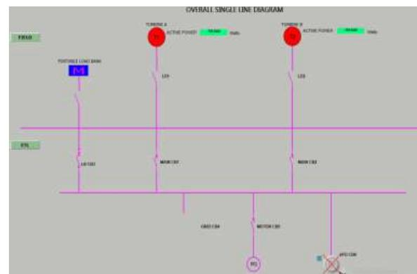
**Figure 1 (b)** MG single line diagram developed in HMI screen used for remote control
