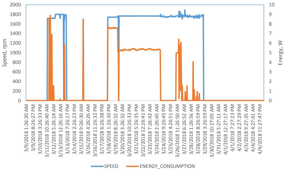
**Figure 9** Condition of a running induction motor: relation between speed and energy consumption
