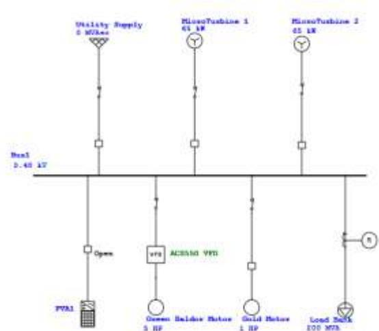
**Figure 1(a).** MG single line diagram used for ETAP simulation
