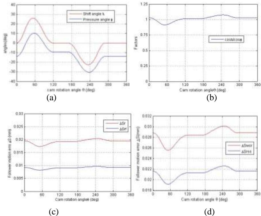
Fig. 12. Mechanical error of cam mechanism with an offset translating roller.
