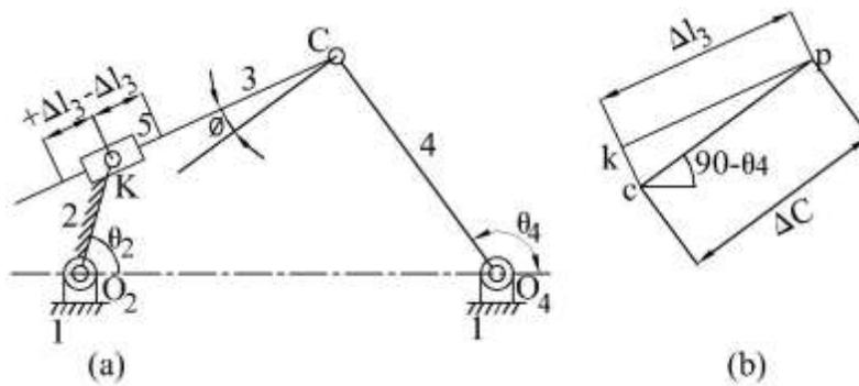
Fig. 9. Substituted equivalent linkage and its smaller displacements diagram
