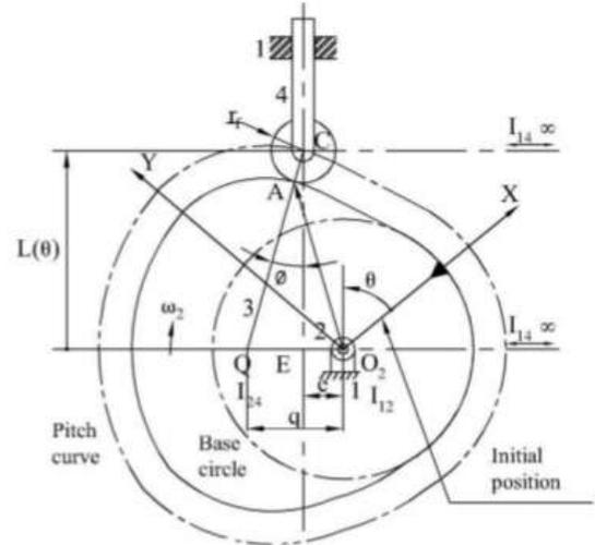
**Fig. 1.** Disc cam with offset translating roller follower
