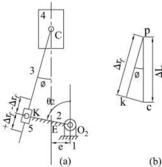
**Fig. 7.** Substituted equivalent linkage and its smaller displacements diagram
