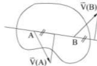
Fig. 3. Vector velocities of point in rigid body
