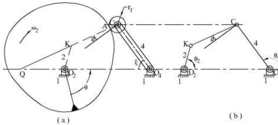
Fig. 8. Cam mechanism and its equivalent linkage
