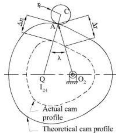
Fig. 11. Actual cam profile and theoretical cam profile
