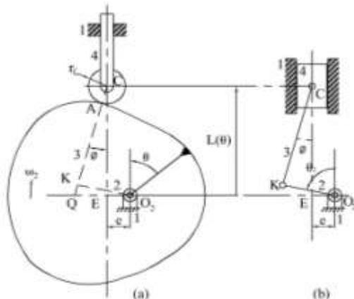
Fig. 5. Cam mechanism and its equivalent linkage
