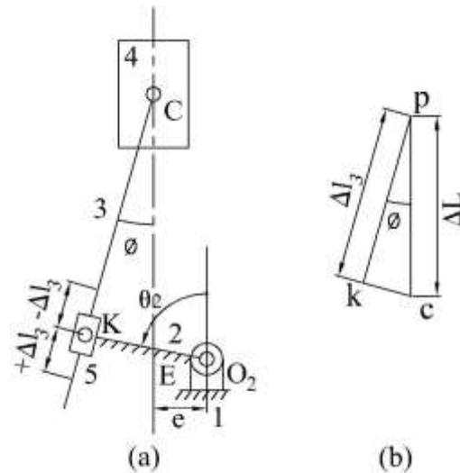
Fig. 6. Substituted equivalent linkage and its smaller displacements diagram
