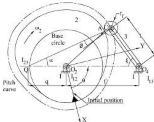
Fig. 2. Disc cam with an oscillating roller follower
