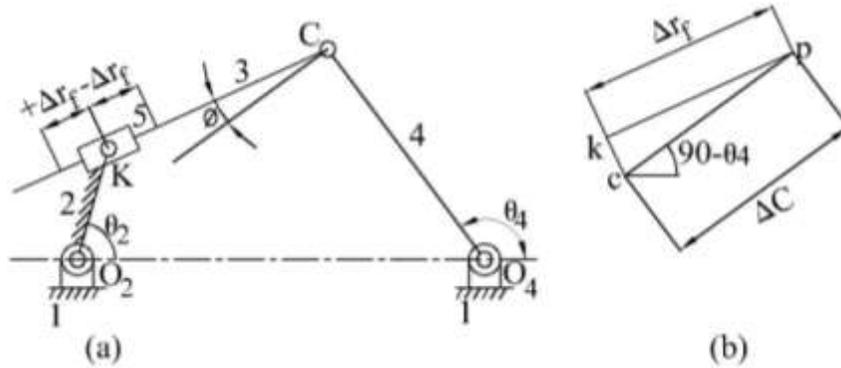
Fig. 10. Substituted equivalent linkage and its smaller displacements diagram
