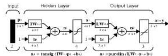
**Figure 1: structure of MLP with hidden neurons and output neurons with linear function**
